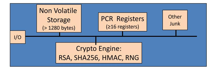
RSA: 1024, 2048 bit modulus SHA256: Outputs 32 byte digest
