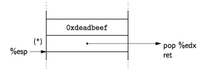
Figure 2: Load the constant **Oxdeadbeef** into **%edx**. From Shacham "The Geometry of Innocent Flesh on the Bone..." 2007
