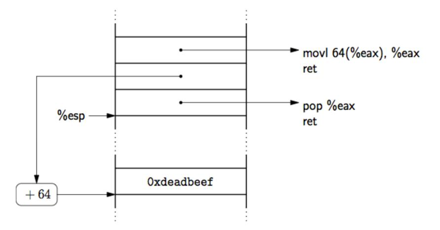
Figure 3: Load a word in memory into %eax.
